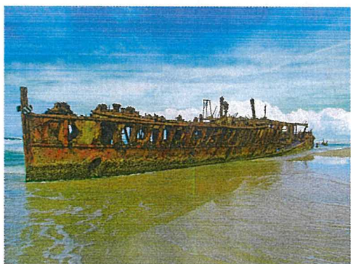
Figure C2.7 ▲ Iron reacts with oxygen and water to form rust – a new compound.
